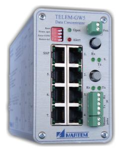
Data Concentrator TELEM-GW5 is used for control and monitoring operations of a system from control center via IEC 60870-5-101, IEC 60870-5-104 data communication protocols and for data collection from lower level peripheral devices and control them using various data exchange protocols IEC 60870-5-101, IEC 60870-5-103, Modbus, Telem.
