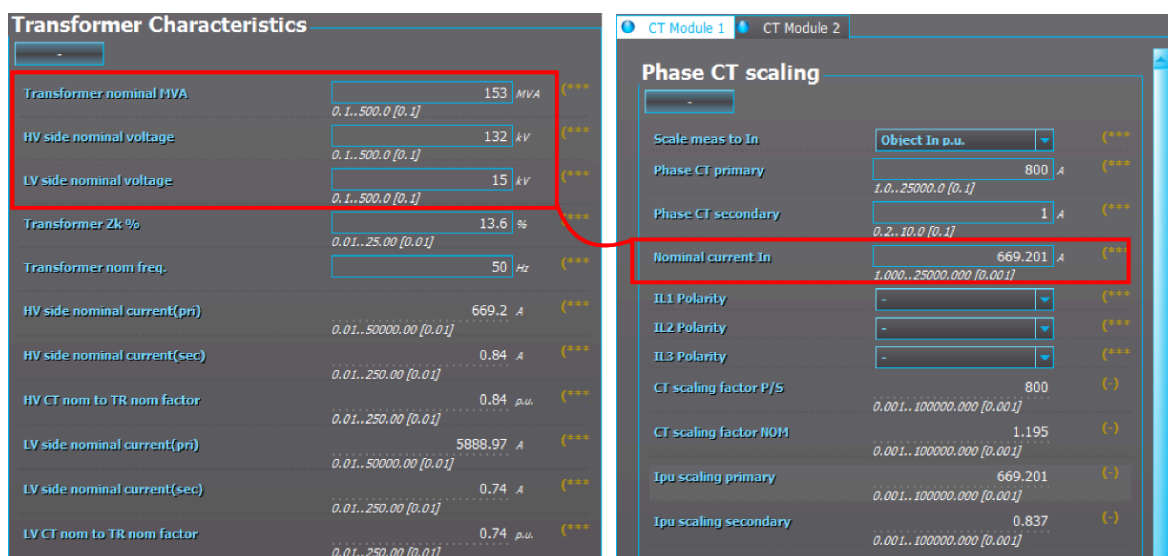
Figure. 5.2.1 - 54. Phase CT scaling to machine nominal.
