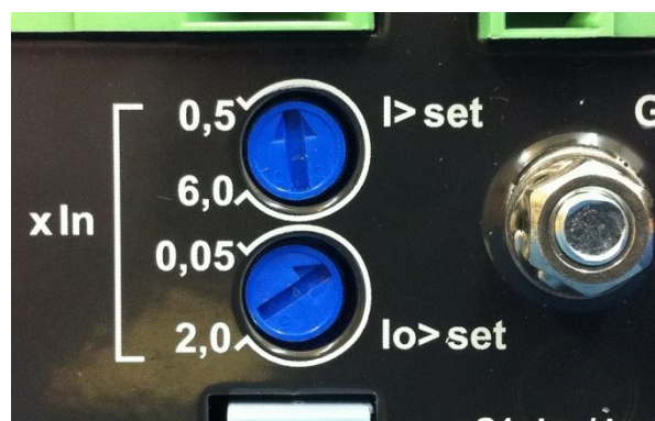
Figure 3-1 AQ110 overcurrent setting trimmers
