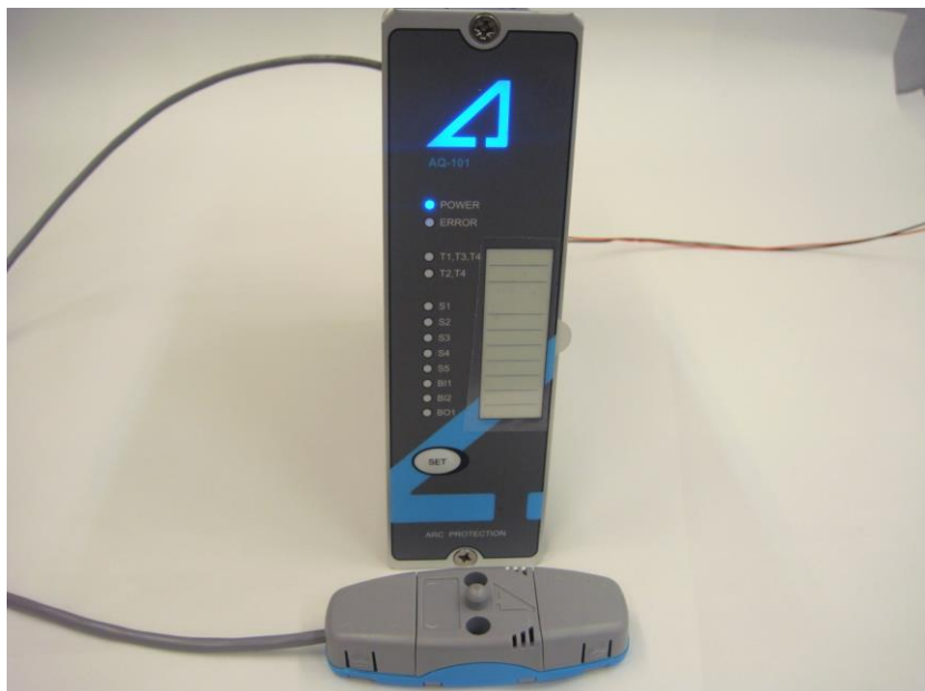
Figure 4-13: AQ01 sensor connection step 8.
